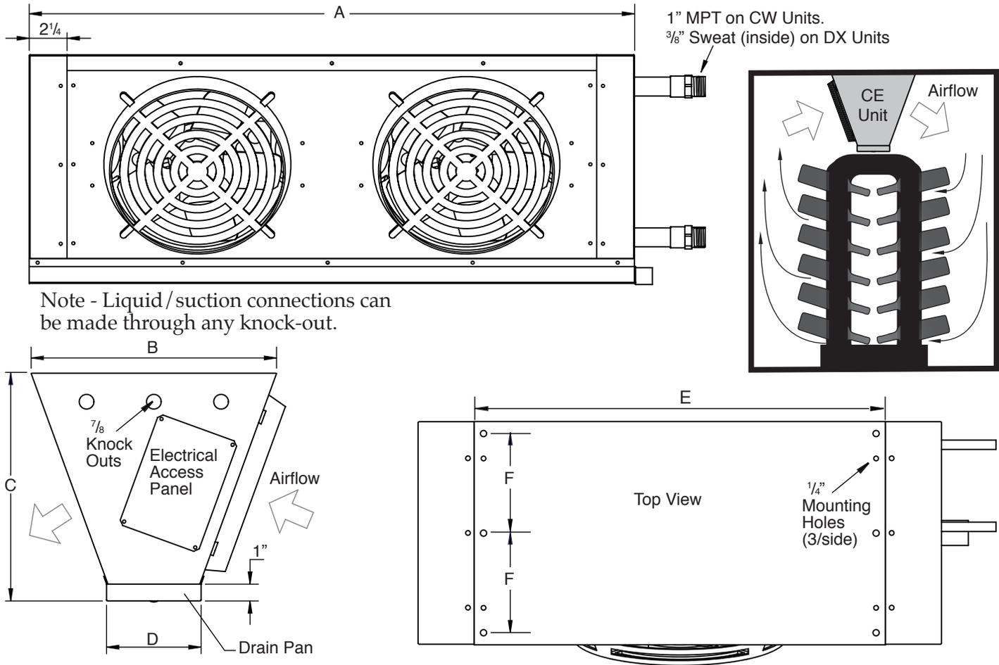
Note - Liquid/suction connections can be made through any knock-out.
