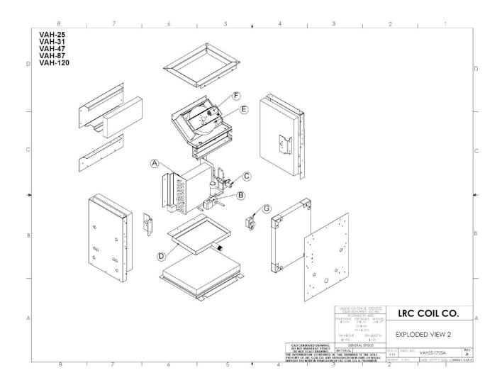
Note: many versions of VAH's have been manufactured up to the time of the introduction of the EC model. With PSC replacement motors getting scarce always get Serial Number for any PSC version and check with engineering.
