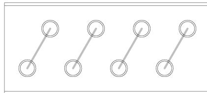
Put a solid dot at the points where a tube comes in or goes out of the coil.
