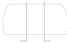
If the brackets stand the coil off the case measure the overall height – the amount the brackets stick out away from the fin pack.
